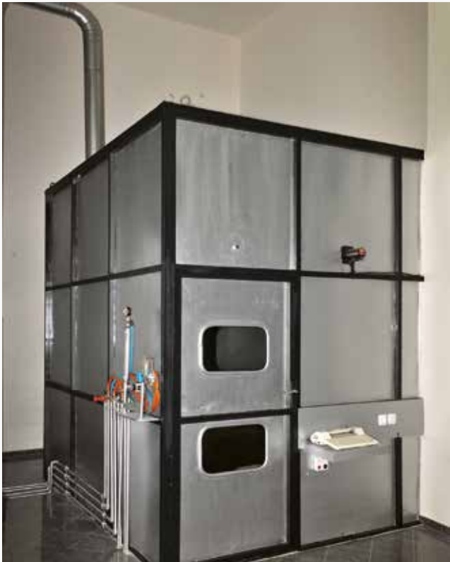
Smoke density testing cabin.
